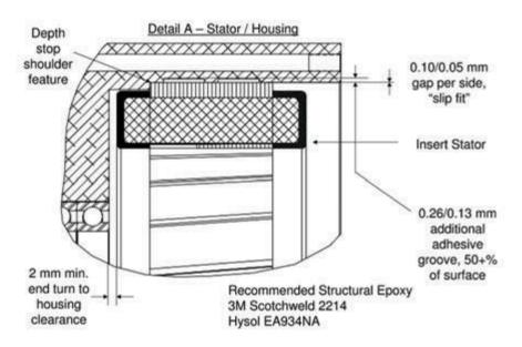
Detail A - Stator/Housing
