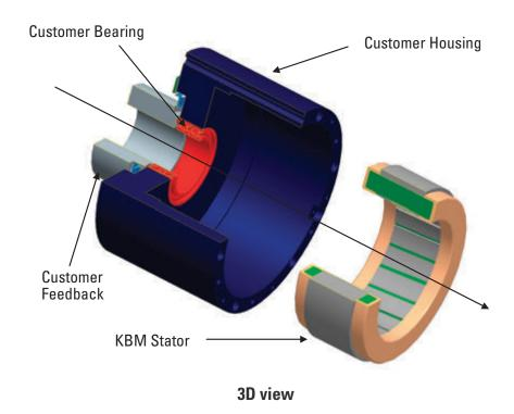
The shoulder serves as a stop point for the stator to bank against when inserted from the open end, and should generally clear the maximum outer diameter of the winding end-turn by no less than 2 mm at all circumferential points. Refer to Detail A.
