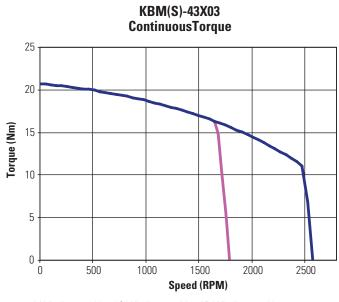
—A Winding-480 Vac / C Winding-400 Vac / D Winding-120 Vac
